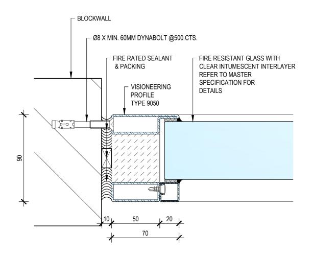
NOMINAL FRL120/120/120 WALL COUNTERSUNK TEK STEEL SCREW MIN. 60MM @500 CTS. FIRE RATED SEALANT & PACKING FIRE RESISTANT GLASS WITH CLEAR INTUMESCENT INTERLAYER REFER TO MASTER SPECIFICATION FOR VISIONEERING **DETAILS** PROFILE TYPE 9050 L HEAVY GAUGE STUD
